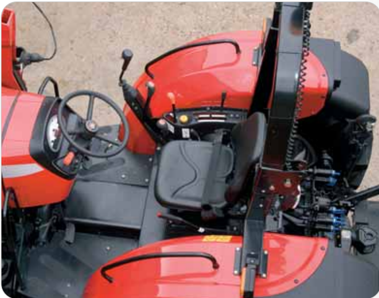
Spacious, semi-platform, with superb controls and 2-post folding ROPS protection
