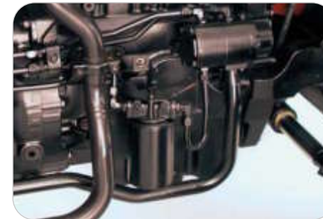
The hydraulic pump for the steering system is externally mounted. Filters are positioned for quick service access.
