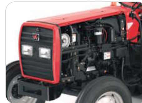
Quickly removable side panels give easy access to air filter, radiator and engine service points
