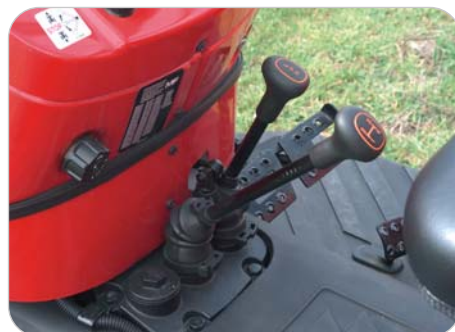
Central gear levers, give a direct, positive gearchange. Note the conveniently placed gearbox oil filler.
