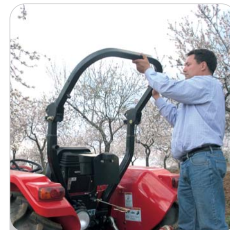
The 2-post safety frame folds easily, for working in low buildings or under overhanging branches
