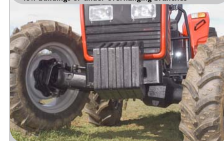
Rugged 4-wheel drive front axle features good ground clearance and a tight, 55° steering angle
