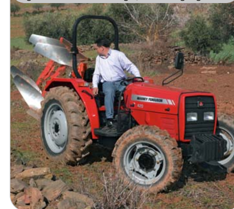
Rugged 4-wheel drive front axle features good ground clearance and a tight, 55° steering angle
