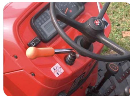
The MF 420 has an 8-speed shuttle gearbox as standard, with a left-hand mechanical lever for forward/reverse selection
