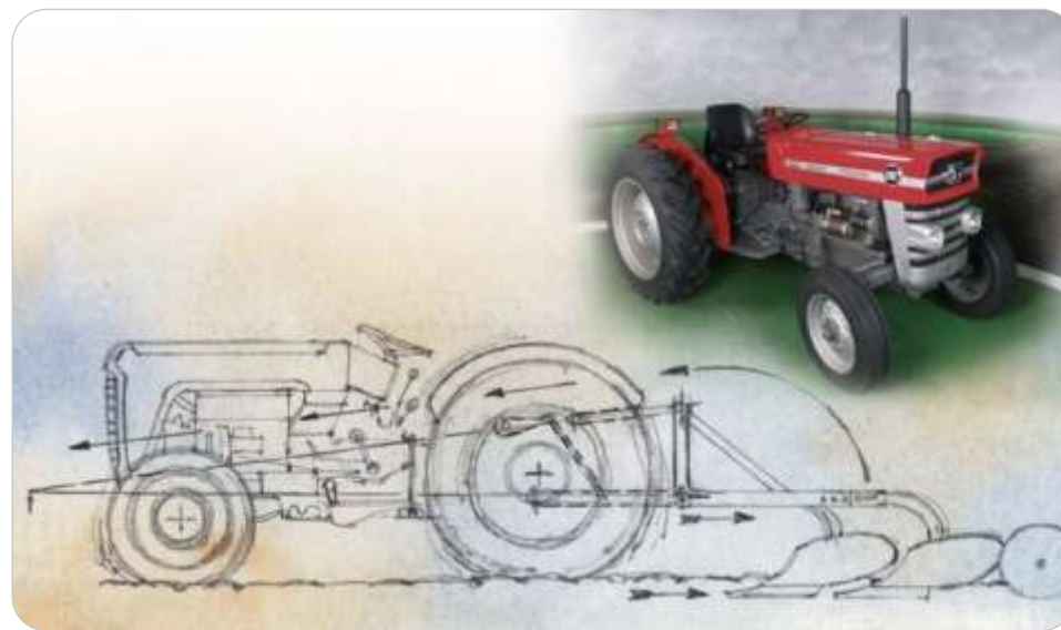
Above: Where it all began. The basic principals of the efficient Ferguson three point linkage
