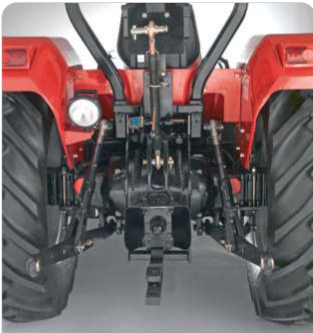
Rugged three point linkage system; simple hydraulic and PTO controls
