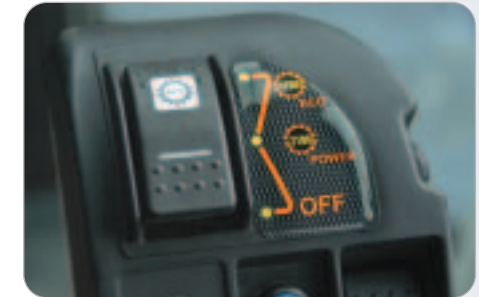
Armrest-mounted control of Speedmatching and AutoDrive modes (Dynashift version)
