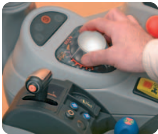
The Autodrive Controller (Dyna-6), can be adjusted to the appropriate setting or moved between sectors at any time, including while operating under load, on-the-move.
