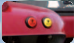
Fender-mounted PTO controls for added convenience and safety
