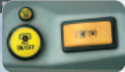
PTO speed selection, engagement and 'Auto' activation switches are well placed and easy to operate
