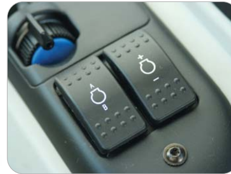
Use '+/-' to pre-set engine speed and 'A/B' to memorise and access the required setting
