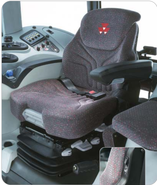
The high specification swivelling seat, featuring armrest mounted controls and seat heating (inset)
