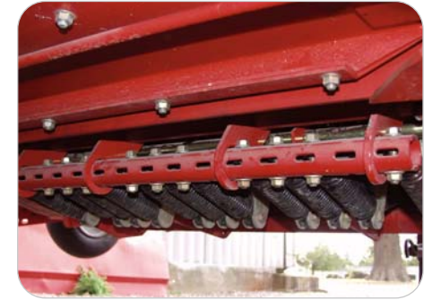
Each cutter knife has its own spring loaded breakaway system to protect against foreign object damage.
