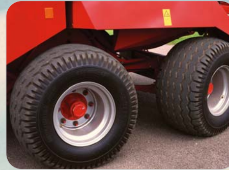
19° of steering angle saves pasture and tyre wear.
