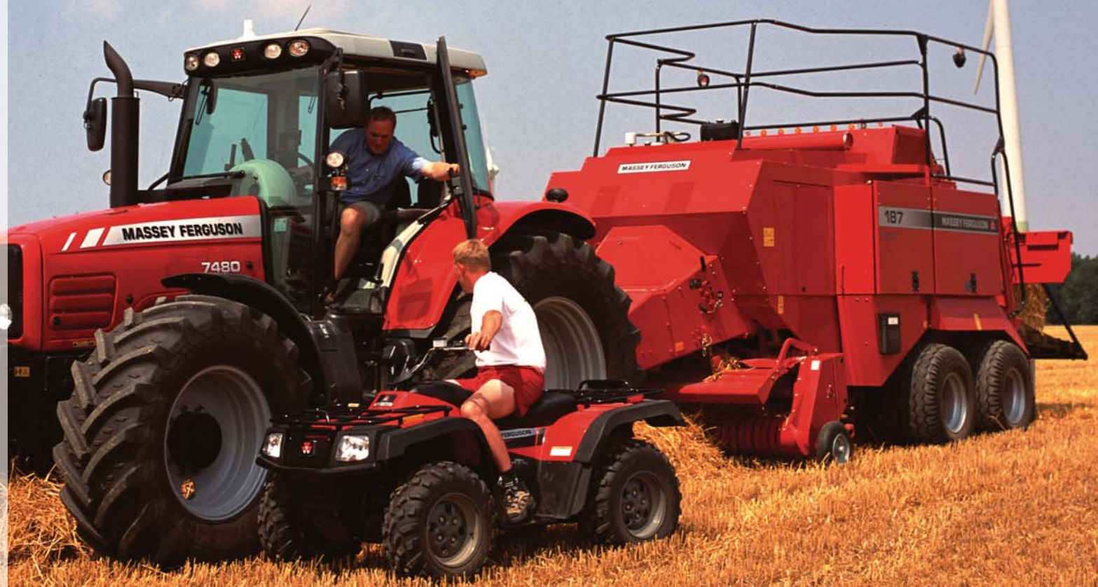
The MF 186 produces bales of 0.70 m x 1.20 m section up to 2.50 m long and will bale silage, hay and straw.
