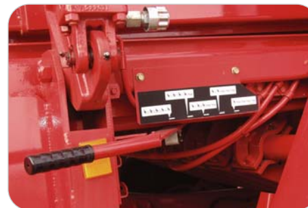
On the MF 185 SII, MF186 and MF 187 the bale ejector lets you remove the last bale or clear the whole chamber. Just select the required number of teeth with this lever.
