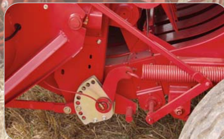
Height adjustment of the pickup is easy using this set plate and pin.
