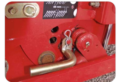
A choice of three preset chop lengths can be easily selected using this selection rod.
