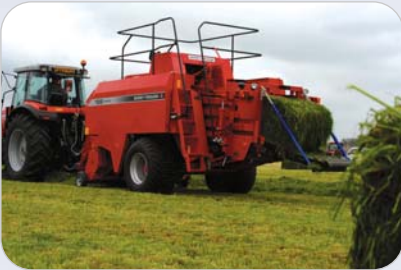
MF185 Series II produces bales of 0.88 m x 0.80 m section up to 2.50 m long and will bale silage, hay, lucerne and straw.
