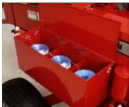
Above: One twine box on each side of the baler gives simple twine routing for more reliable tying
