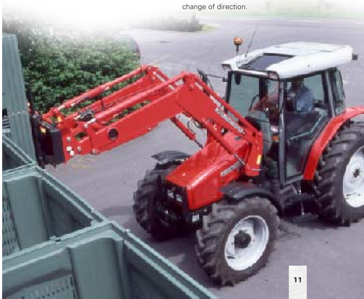
Right: The electronically controlled clutch on PowerShuttle models can be used as an 'inching pedal' - ideal for precise loader work. ('Visi-Roof' cab option shown)
