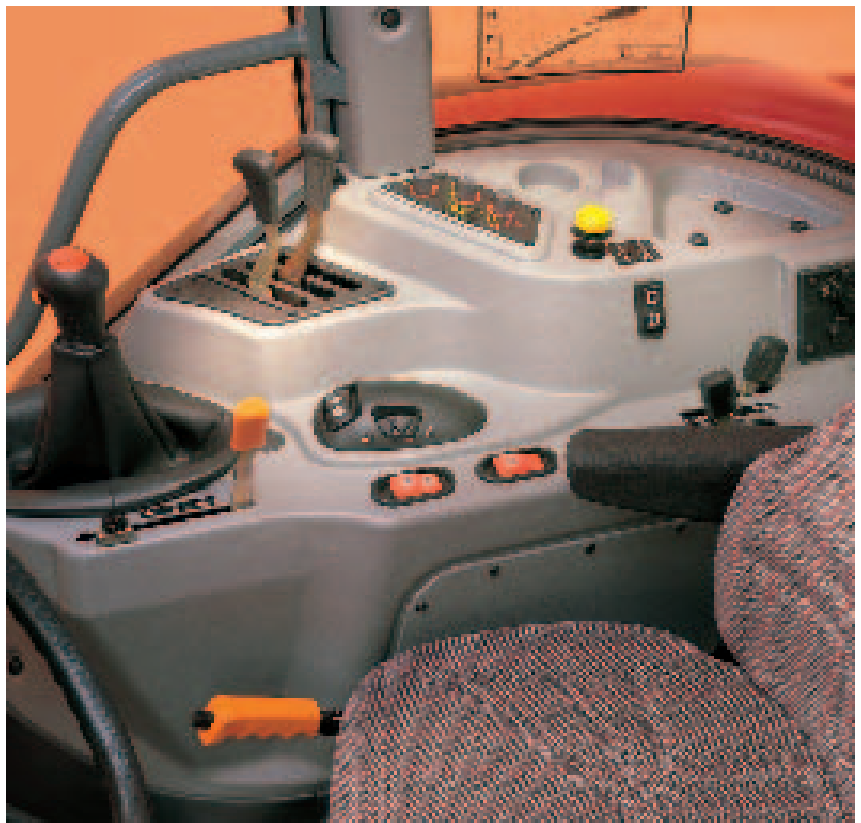
Right: Superb new right-hand console. Gear lever is angled to follow natural arm movement (Model shown has optional Electronic Linkage Control)
