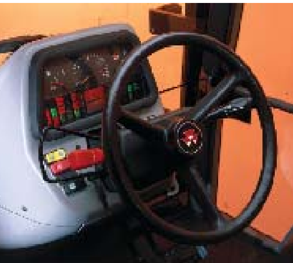
Above: Instrumentation is clear and concise. Digital readouts* give accurate PTO and forward speed (*depending on specification)
