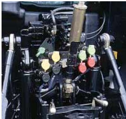
Left: Electrospools shown, on optional CCLS system
