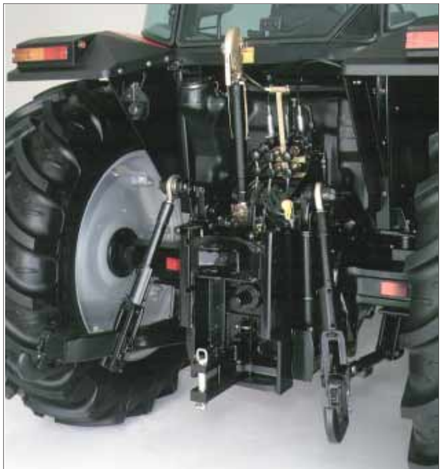
Left: Electrospools shown, on optional CCLS system
