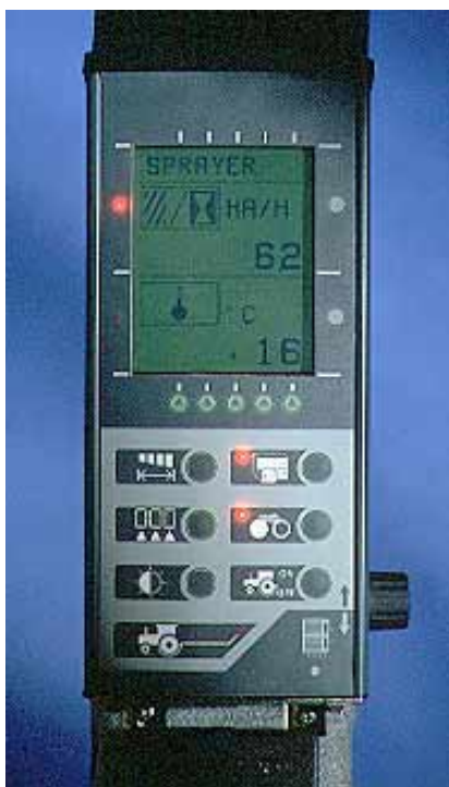
Datatronic II (optional) has over 20 functions and twin digital displays
