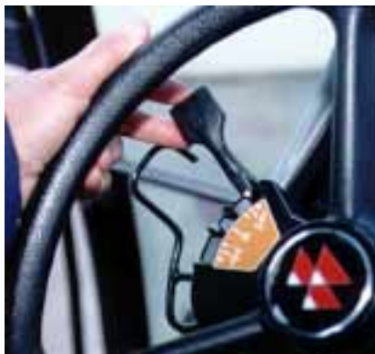
Left: The Multi-function Power Control lever operates as on Dynashift Plus models - fully described on Page 10
