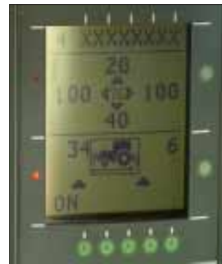
Right: Timing of front and rear equipment entry and exit can be set via the Datatronic II monitor
