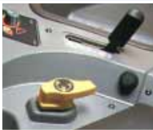
Large, safe, simple PTO controls
