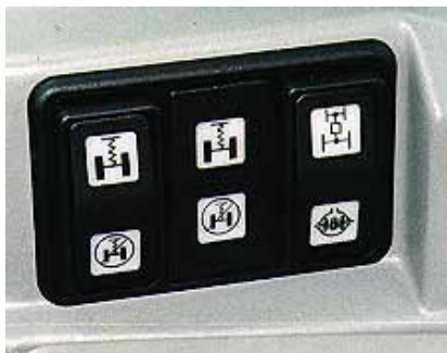
Left: Simple engagement and disengagement of front suspension and front differential lock
