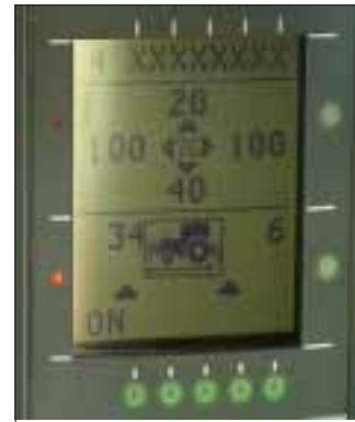
Right: Timing of front and rear equipment entry and exit can be set via the Datatronic II monitor
