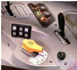
The PTO is actuated by large rotary switches. (Optional) In-cab shifttable PTO lever and QuadLink controls also shown.
