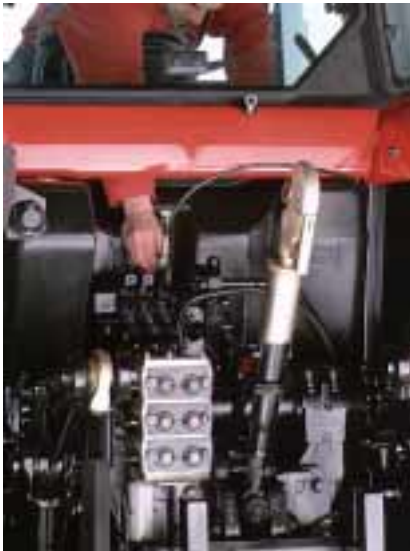
Lever-action couplers mean easy connection and disconnection, even when pressurised. Each mechanical spool valve has individual, flow control from the driver's seat.
