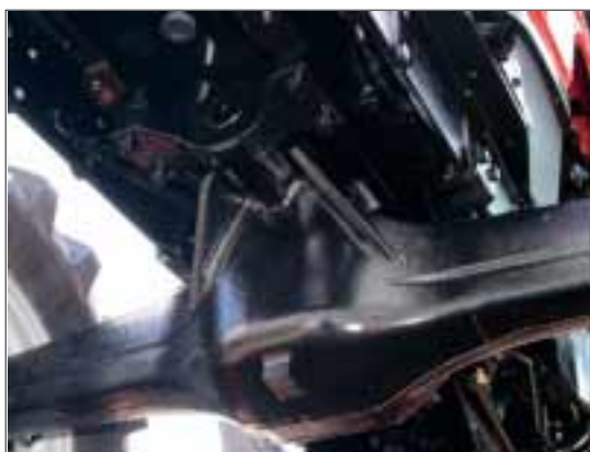
Above: All 8200 models now feature 'high pivot' design and Hydra-lock differential
