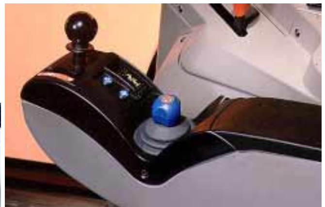
Speed selection is either via the Power Control lever or the armrest control (Powershift models)
