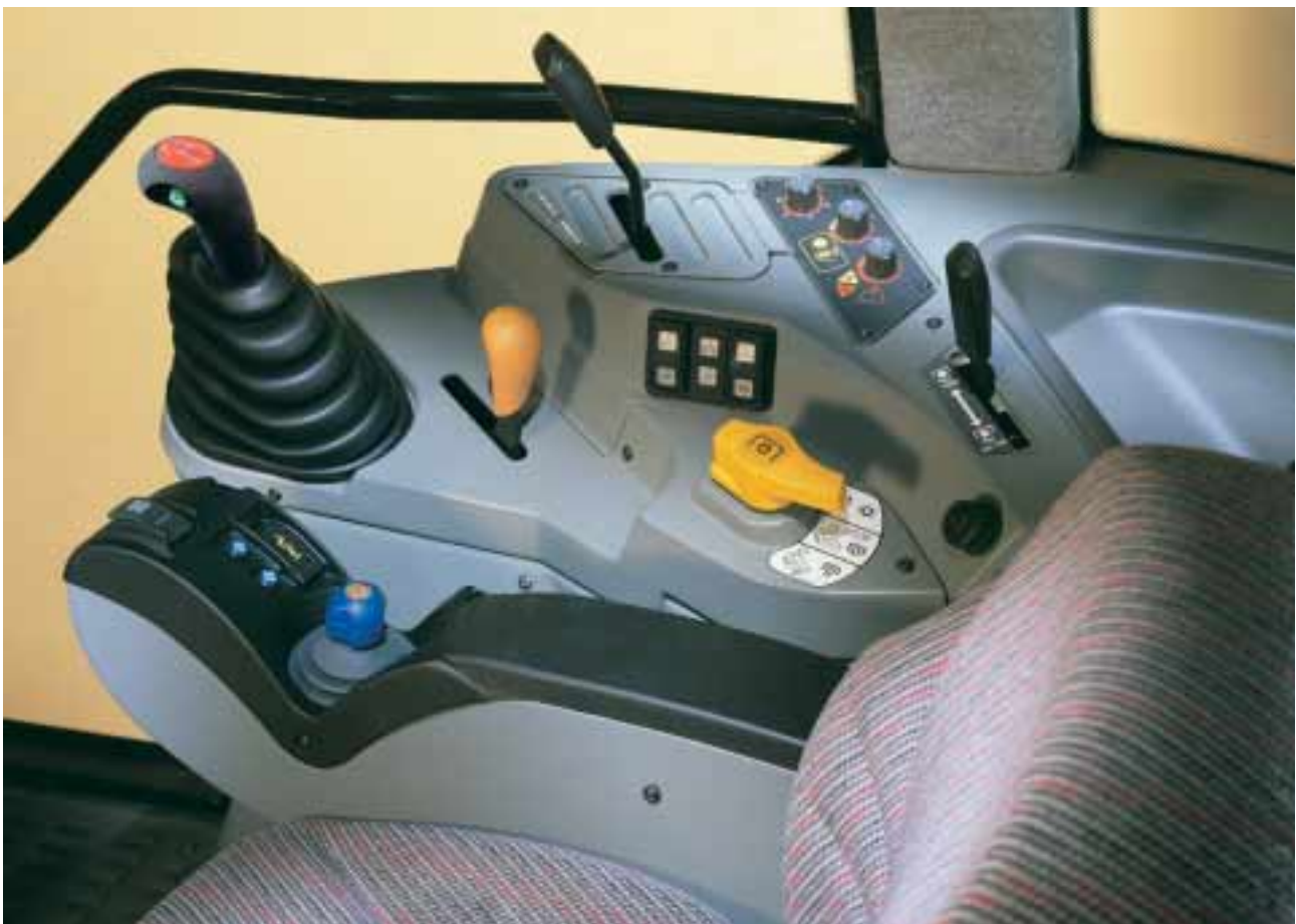
Right and below: Layout includes convenient armrest mounted controls (Dynashift model shown with optional SMS 'joystick' spool valve control).
