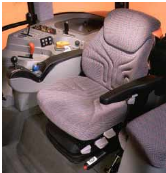
Left: The high specification swivelling seat, featuring armrest mounted controls (optional SMS and QuadLink controls shown)
