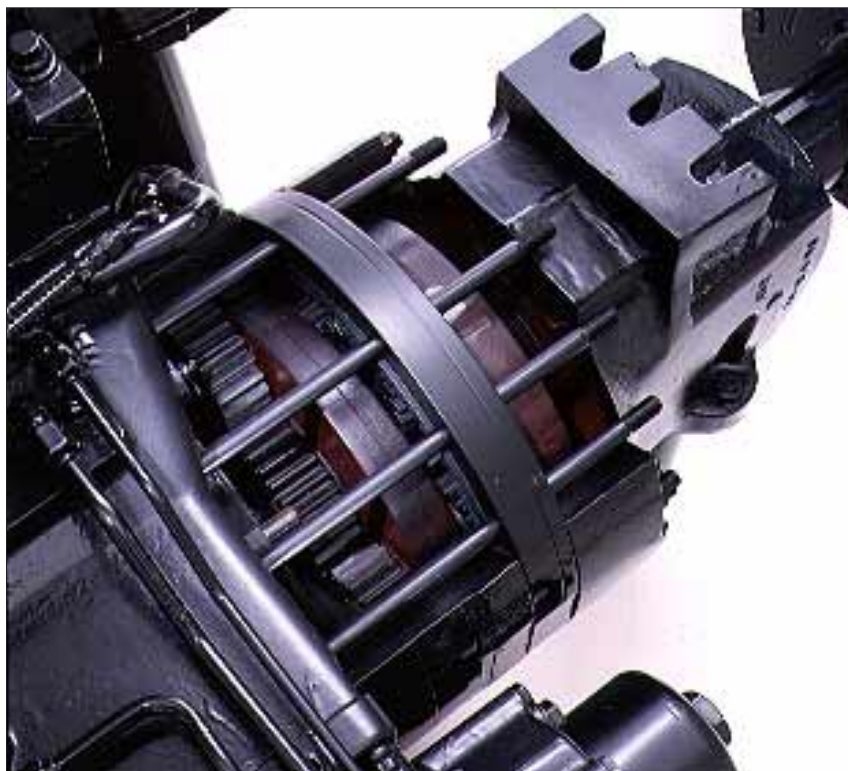
Right: The massive rear axle (MF 8270/8280 shown) features large oil immersed disc brakes and heavy duty inboard dual epicyclic reduction units ensuring strength, safety and durability.
