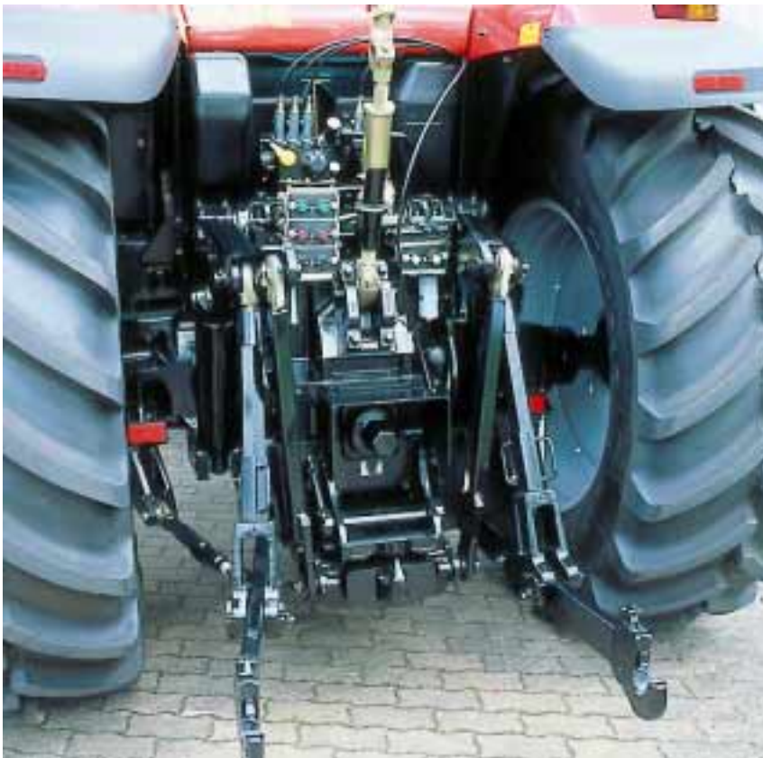
Below: Linkage and hydraulic specifications are available to suit all market needs and legislation. (MF 8220, UK specification shown, below)
