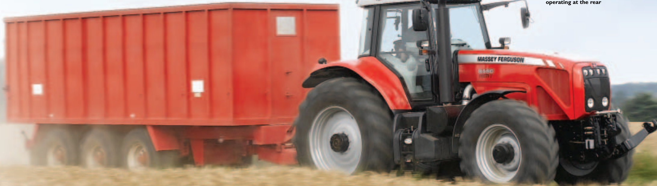
The cab is flexibly mounted at the front, with the 'Dual stage' cab suspension system operating at the rear
