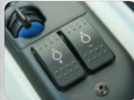
Use '+/-' to pre-set engine speed and 'A/B' to memorise and select the required setting
