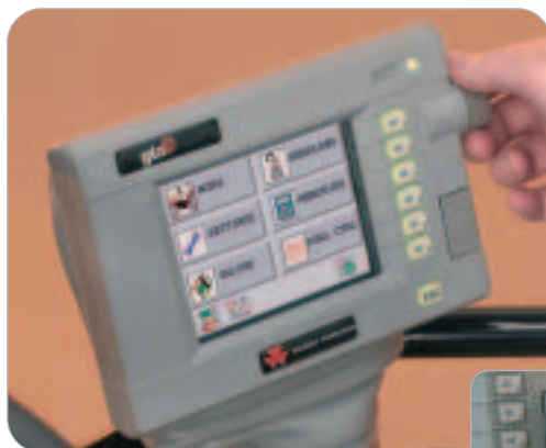
GTA Console makes settings and adjustments easy. Legibility is good in all ambient light conditions. Inset: SD memory card slot for data transfer
