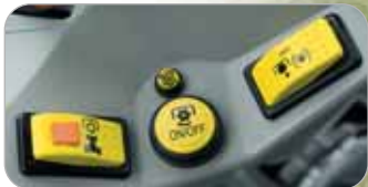
PTO speed selection, engagement and 'Auto' activation switches are well placed and easy to operate
