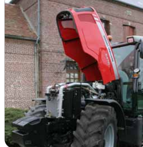
Above: New hinged bonnet design gives excellent service access on 4-cylinder models
