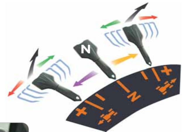
Power Control enables forward/reverse shuttle, powershift changes and fingertip de-clutching - all from a single, convenient lever
