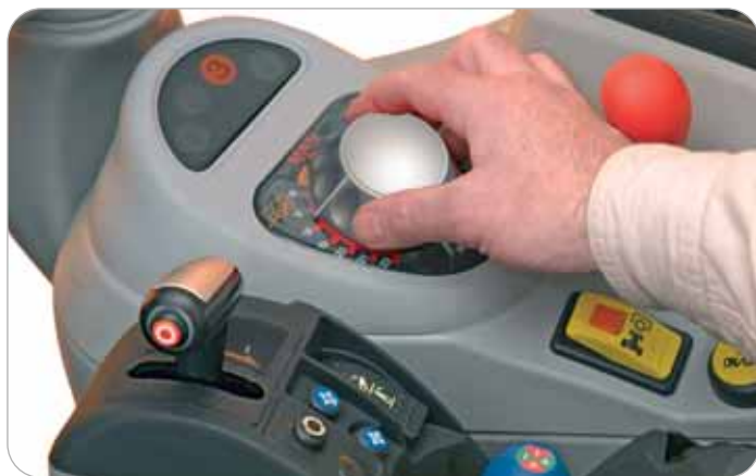
The Autodrive Controller can be adjusted at any time to achieve ideal transmission settings to suit varying conditions and applications
