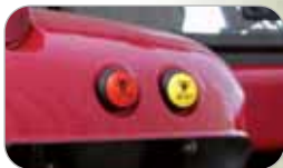
Fender-mounted PTO controls for added convenience and safety
