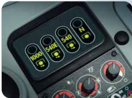
Fender-mounted PTO controls for added convenience and safety
