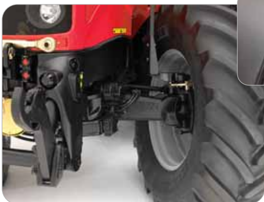
New 'waisted' front support casting design enables a tight turning angle
