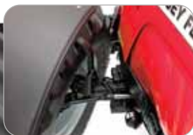
New 'waisted' front support casting design enables a tight turning angle
