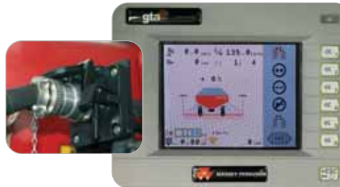
Typical ISOBUS screen image inset: implement connection
