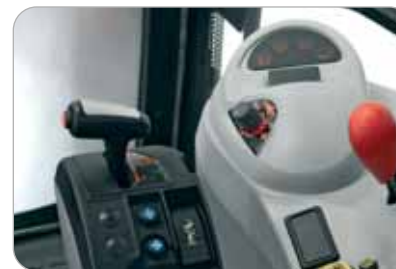
Above: Dyna-6 'T-handle' gear lever with Speedmatching and forward/reverse shuttle 'Comfort Control'
