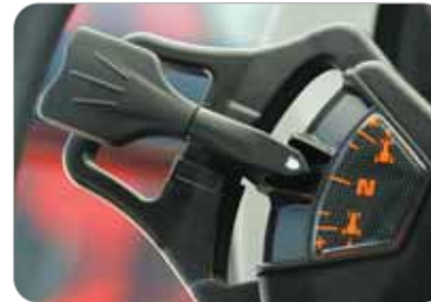
Power Control enables forward/reverse shuttle, powershift changes and fingertip de-clutching - all from a single, convenient lever
