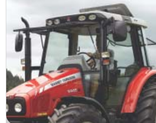
The optional opening front screen gives extra ventilation
