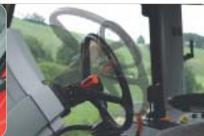
Available as an option, a single lever controls adjustment of steering column height and tilt
