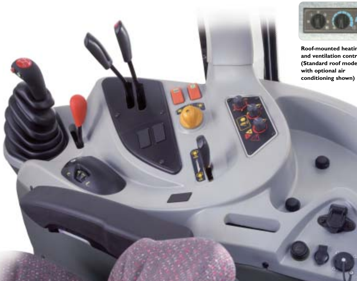
Other ELC functions are set by smooth, rotary controls. LEDs indicate linkage lifting and lowering.
