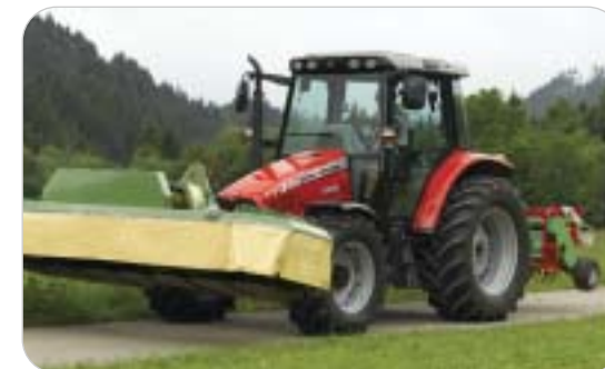
Above right: Integrated Active Transport Control (ATC) gives faster, safer transport of mounted equipment
