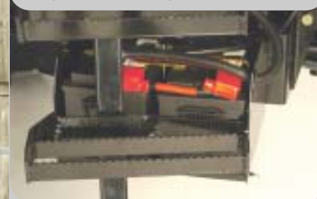
Remove a cover for fast battery access
