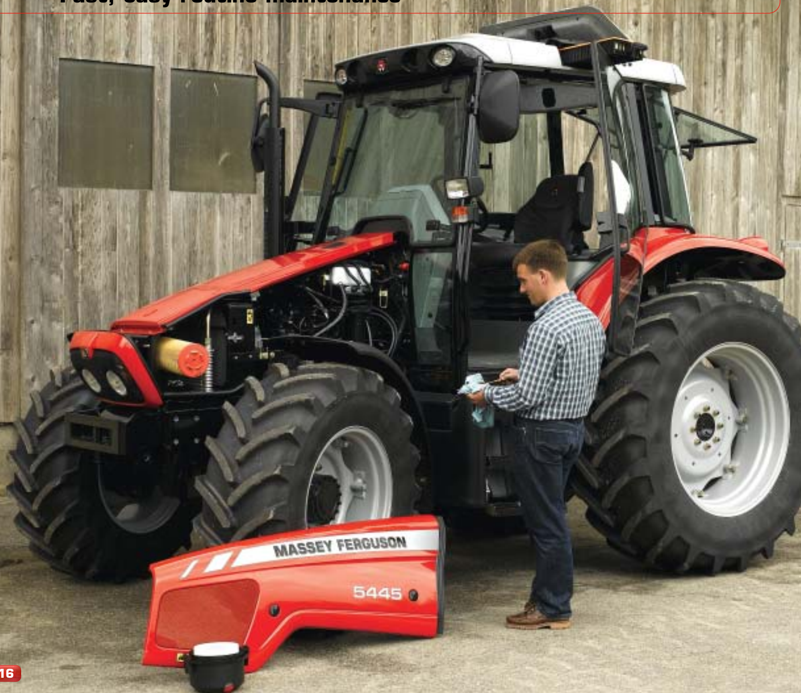
Easy access to dual, dry air cleaner
