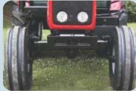
Left: Both 2- and 4-wheel drive front axles have excellent ground clearance and turning angle
