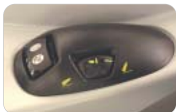
The ELC 'mouse' fits naturally in the hand, giving comfortable control of linkage lift height
