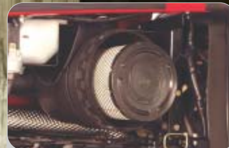
Easy access to dual, dry air cleaner
