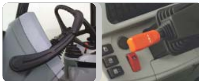
Single lever gear selection with convenient buttons for 'powershift' and range change
