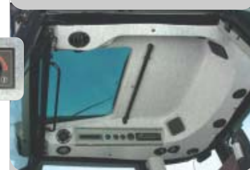
Visio roof models have side-mounted radio (optional) and ventilation controls
