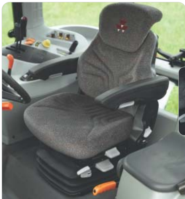
Left: Both mechanical and air suspended seats (shown) swivel and have a wide range of adjustments
