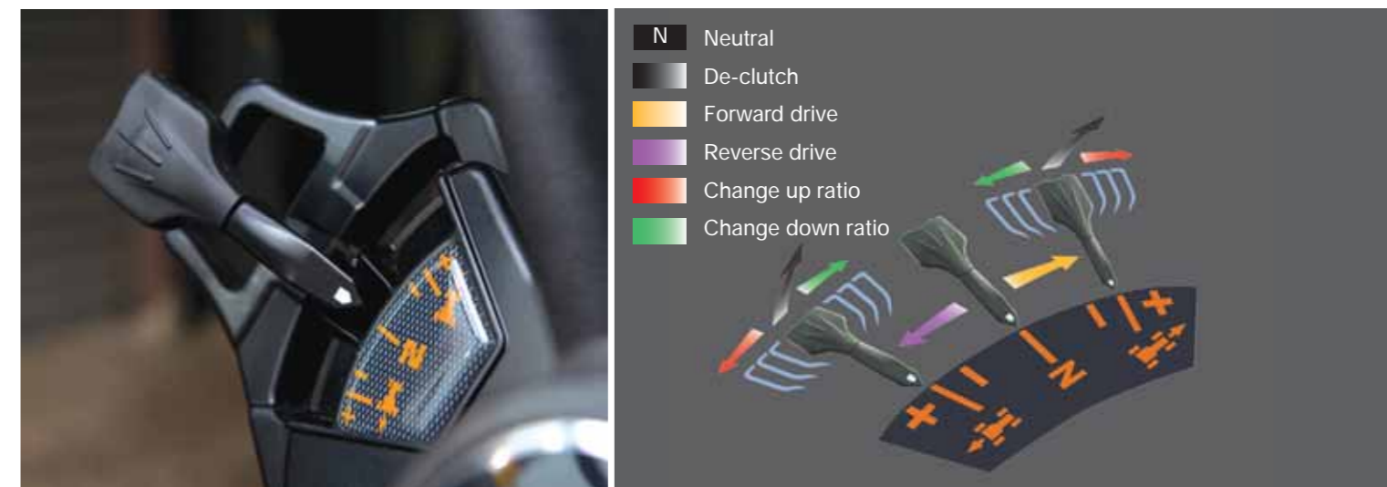
Power Control lever The left-hand Power Control lever provides convenient and straightforward operation. From here you can operate forward/reverse shuttle, powershift and range changes and fingertip de-clutching, leaving the right hand free to operate the loader or rear implements.
