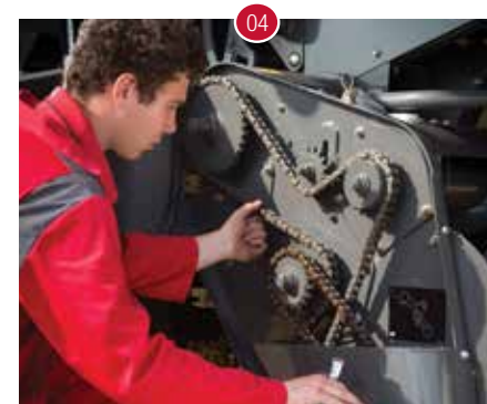
Checking the pick-up chain tensions.
