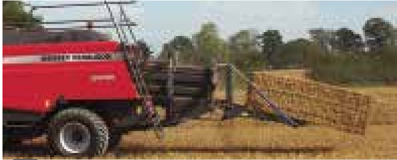
The Integrated Bale Weighing System weighs the bale as it exits the chamber onto the roller bale chute.
