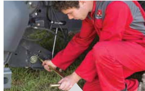
Three pre-set chop lengths can be easily selected using this selection rod.
