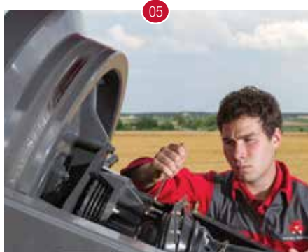
Adjusting the flywheel slip clutch.
