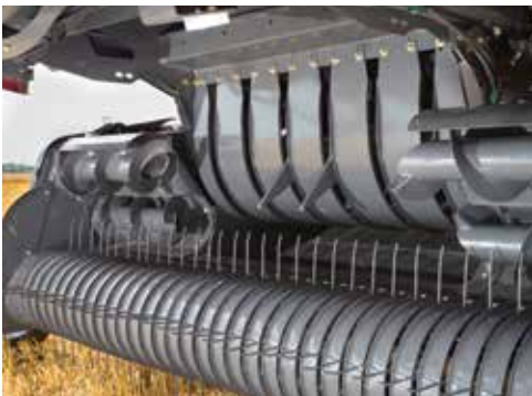
Four 'Quad' augers ensure higher capacity feed on 'Packer' balers.
