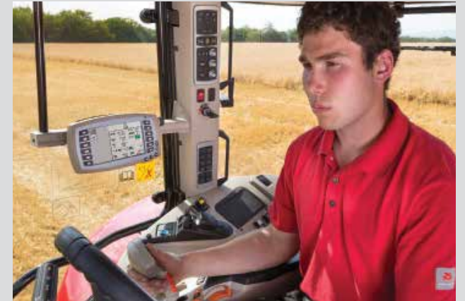
Controlling the baler via the tractor ISO VT terminal.
