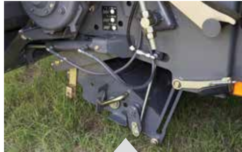
Lowering of the knife bed gives easy access to the knives and aids removal of foreign objects.
