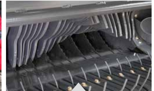
Heavy duty four-lobed spiral cutter rotor for smooth crop flow.
