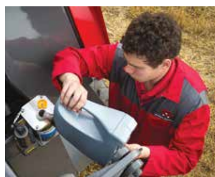
Refilling the automatic chain oiler.
