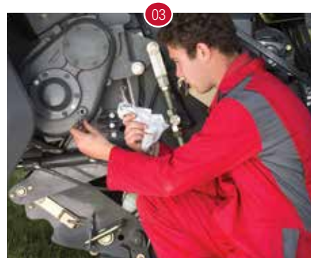
Checking the cutter gearbox oil level.
