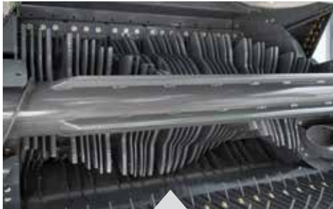
Heavy duty cutter rotor with full width powered feed auger.
