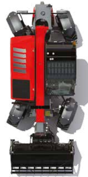
Four-wheel steering mode - for minimum turning circles.
