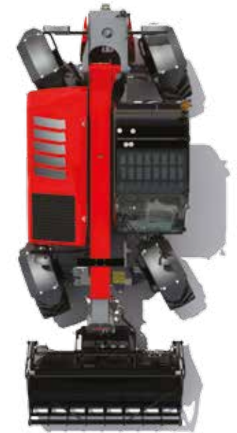
Crab-steer mode - for efficient filling and grading and working alongside walls and in confined spaces.
