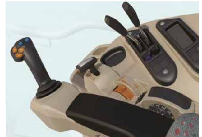
The MF 5700 SL Essential cab option with loader electronic multifunction joystick
