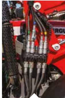
Base configuration with flat faces single couplers
